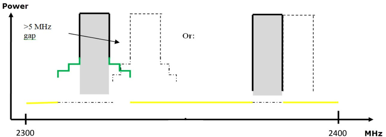
Figure 3: Combined BEM elements for adjacent blocks with unsynchronised TDD networks
